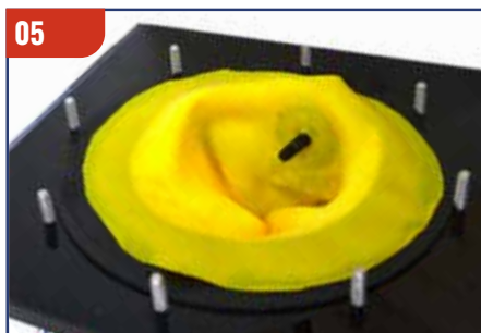
FLATTEN PALPATION LINER AGAINST WASHER
